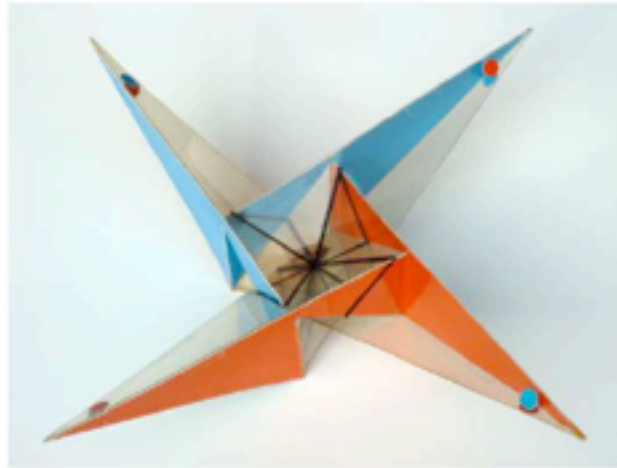
Fig. 9 Open halfway model: handmade models need ability, precision and perseverance. The pentagons are obtained by gluing together two cardboard sheets – one side in red for the one and one side in blue for the other. To work the rhodoïd, a steel edge and a fine cutter are necessary. To mark the rhodoïd from the plans, needles and a small hammer were used. Faces are fixed together with adhesive tape. The self-intersection line is drawn by using a pencil with permanent ink.
